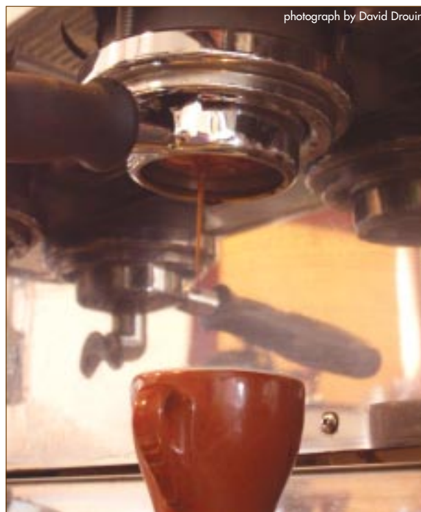
Use of a bottomless portafilter allows baristas to troubleshoot their technique.
